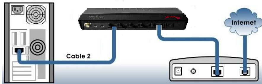
RNX-N400LX, PC, and Modem Rear View (WAN Port and LAN port Connection diagram between PC, Wireless Router and Modem)
