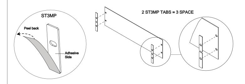
NOTE: When using two (2) ST3MP Shim Tabs, ensure that the holes in the Shim Tabs align with the mounting holes on the component.
