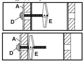
Pull screw ( $\mathbf{D}$ ) back until toggler ( $\mathbf{E}$ ) hits the inside of the metal stud. Fasten all six screws ( $\mathbf{D}$ ) tight, until wall plate ( $\mathbf{A}$ ) is flush with wall.
