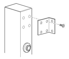
Attach the Rack PDU to a vertical mounting rail in the rear of the enclosure using two additional screws per bracket (not provided).
