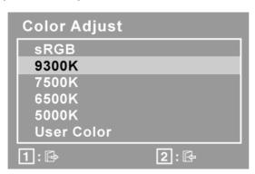
**sRGB-**This is quickly becoming the industry standard for color management, with support being included in many of the latest applications. Enabling this setting allows the LCD display to more accurately display colors the way they were originally intended. Enabling the sRGB setting will cause the Contrast and Brightness adjustments to be disabled.
