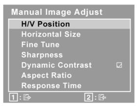
**H./V. Position (Horizontal/Vertical Position)** moves the screen image left or right and up or down.
