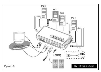
This section describes how to connect the computer(s) you wish to control, to the KVM switch.
