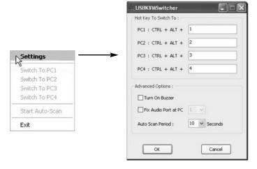
From within the KVM Switcher software, you also have the option to fix the audio/mic channel to the selected PC. Once this option is check, the audio/mic channel will be fixed and become non-switchable without re-configuration.
