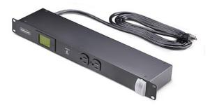
This 1U Rack Mount Metered PDU features a built-in 8ft (2.4m) NEMA 5-15P power cord and 8x NEMA 5-15R outlets, while the surge protection helps ensure the safe and stable operation of critical equipment. A large backlit LCD provides live readings of electrical parameters for connected devices.
