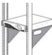
Flush mounting (RS500 & RS700)
