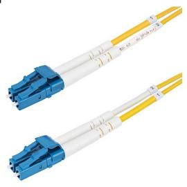
OS2 LC to LC Single Mode Duplex Fiber Optic Patch cable facilitates connectivity across 100G networks. It supports Coarse Wavelength Division Multiplexing (CWDM) across an extended wavelength range of 1260-1625nm, improving channel isolation for optimal signal strength over long distances.
