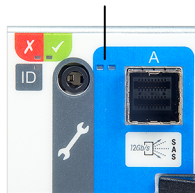
Figure 2-9 I/O module SAS Activity LED location
