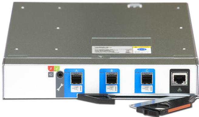
Figure 2-6 Veritas U12 65.5TiB/72TB Storage Shelf I/O module
