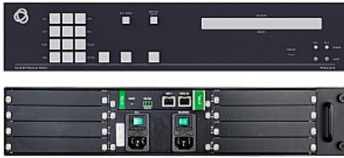
MTX3-16-M is an intelligent and high performance 16x16 modular matrix for switching and distribution of multi-format audio-visual signals. The chassis includes a CTRL central control card with secured LAN connectivity for remote management and control, and has eight card slots for flexible insertion of modular matrix cards, accommodating matrix cards with quad or dual ports of either input or output multi-format signals
