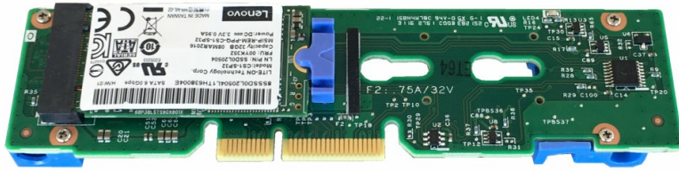
Figure 12. ThinkSystem M.2 Enablement Kit (shown with an 32 GB M.2 drive, not supported in the SE350)
