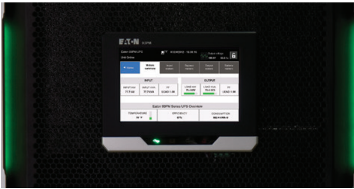
Green light bars showing healthy UPS.
