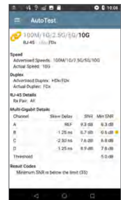
Cabling SNR measurement validates Multi-Gig links
