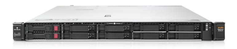
The HPE Aruba Networking EdgeConnect SD-WAN EC-XL-H is a 1 U rack-mountable hub gateway platform that serves to build an SD-WAN fabric using zero touch provisioning. It supports-MPLS, 4G/LTE/5G and internet-based hybrid WAN transport services and a control plane that is automated and secured by the HPE Aruba Networking SD-WAN Orchestrator centralized management software providing policy-based virtual network segmentation and acceleration of on-premises and SaaS cloud applications.
