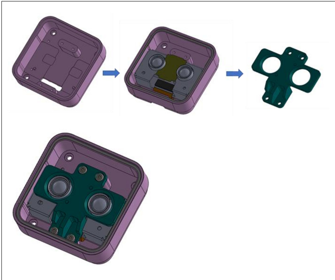
Figure 7-15. Stereo Depth Module Mid-Mounting – D401
