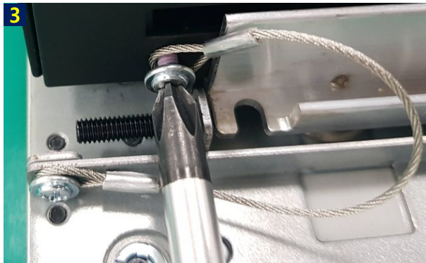
Using M3, L6 BH screw Fixing Safety Wire and BRACKET-FRAME
