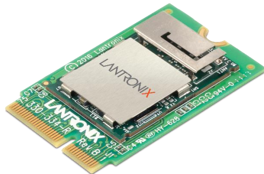
XPC2404 – Edge Connector, On-Module Antenna
