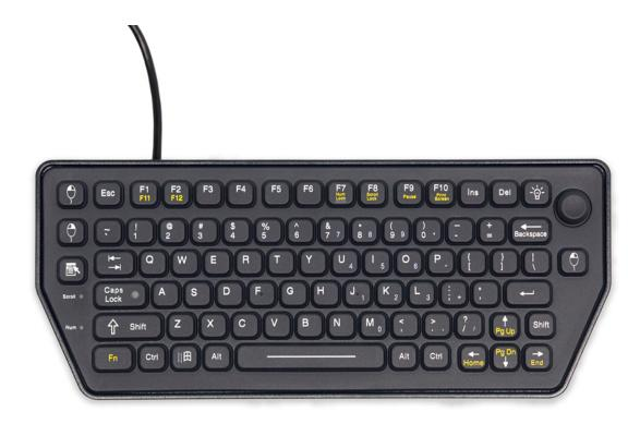
Featuring an integrated Force Sensing Resistor pointing device with dual left-click capability, the SLK-79-FSR offers a large amount of functionality in an ultra-small package. For working in low-light environments, the SLK-79-FSR features the added convenience of backlit keys. Like other keyboards in the iKey line, the SLK-79-FSR features sealed industrial silicone rubber keypads, as well as robust ABS polycarbonate cases.
