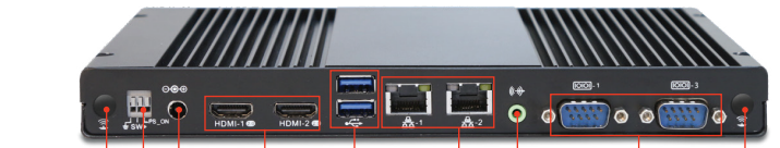
Antenna Hole DC-in USB 3.0 x 2 LAN x 2 Line-out COM port x 2 Antenna Hole
