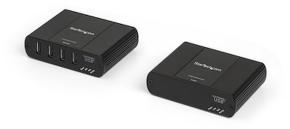
The 4-Port USB 2.0 over Ethernet Extender lets you extend USB devices over a Gigabit Ethernet Local Area Network (LAN) using dedicated Cat5e, Cat6, or Cat7 cabling up to 330ft (100m).
