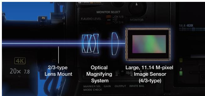
The AJ-CX4000GJ has the Panasonic original optical magnifying system, same as the AK-UC4000 4K studio camera having good reputation for its image quality. If designed 4K image sensor with a 2/3-type size, the pixel size is reduced from the 5.0 microns of HD to 2.5 microns, thereby lowering the image quality and sensitivity. An optical magnifying lens allows the mounting of a large sensor on a 2/3-type lens mount.
