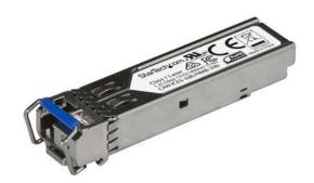
The SFPGE40KT3R5 is a Juniper SFPP-10GE-SR compatible fiber transceiver module that has been designed, programmed and tested to work with Juniper brand switches and routers. It delivers dependable 1 GbE connectivity over fiber cable, for 1000Base-BX40-U compliant networks, with a maximum distance of up to 40 km (24.8 mi).
