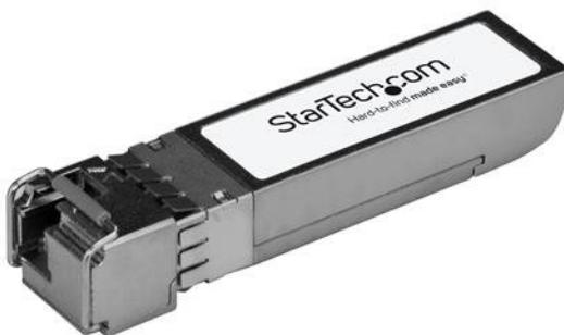
The SFP-10G-BX60U-I-ST is a Cisco SFP-10G-BX60U-I compatible upstream fiber SFP+ transceiver which pairs with StarTech.com's SFP-10G-BX60D-I-ST. They are designed, programmed and tested to work with 10GBase-BX compatible Cisco switches and routers. The SFP+ transceiver module supports a maximum distance of up to 60 km (37.3 mi) and delivers dependable 10 GbE connectivity over fiber cabling.
