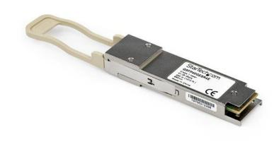
The QSFP-40G-SR4-S-ST is a Cisco QSFP-40G-SR4-S compatible fiber transceiver module that has been designed, programmed and tested to work with Cisco brand switches and routers. It delivers dependable 40 GbE connectivity over fiber cable, for 40GBase-SR4 compliant networks, with a maximum distance of up to 100 m (328 ft).
