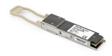
The JG325A-ST is a HP JG325B compatible fiber transceiver module that has been designed, programmed and tested to work with HP brand switches and routers. It delivers dependable 40 GbE connectivity over fiber cable, for 40GBase-SR4 compliant networks, with a maximum distance of up to 150 m (492 ft).
