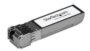
The JD094B-BX-U-ST is an HP JD094B-BX-U compatible upstream fiber SFP+ transceiver which pairs with StarTech.com's JD094B-BX-D-ST. They are designed, programmed and tested to work with 10GBase-BX compatible HP switches and routers. The SFP+ transceiver module supports a maximum distance of up to 10 km (6.2 mi) and delivers dependable 10 GbE connectivity over fiber cabling.
