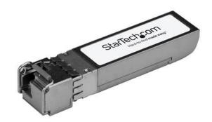
The JD094B-BX-D-ST is an HP JD094B-BX-D compatible downstream fiber SFP+ transceiver which pairs with StarTech.com's JD094B-BX-U-ST. They are designed, programmed and tested to work with 10GBase-BX compatible HP switches and routers. The SFP+ transceiver module supports a maximum distance of up to 10 km (6.2 mi) and delivers dependable 10 GbE connectivity over fiber cabling.
