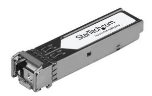
The 10056H-ST is an Extreme Networks 10056H compatible downstream fiber SFP transceiver which pairs with StarTech.com's 10057H-ST. They are designed, programmed and tested to work with 1000Base-BX-D compatible Extreme Networks switches and routers. The SFP transceiver module supports a maximum distance of up to 10 km (6.2 mi) and delivers dependable 1 GbE connectivity over fiber cabling.
