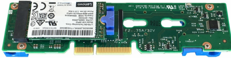
Figure 3. Single M.2 Adapter and a 32 GB M.2 drive
