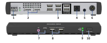
**DXZC-EM front and rear view. 1** Network port. **2** DisplayPort connectors. **3** USB ports (two for high charge-current devices). **4** Feature connector socket. **5** Line-level audio output. **6** DC power inlet. **7** Mic and headset sockets. **8** Easy access USB. **9** LED indicators. **10** Power/Menu switch.
