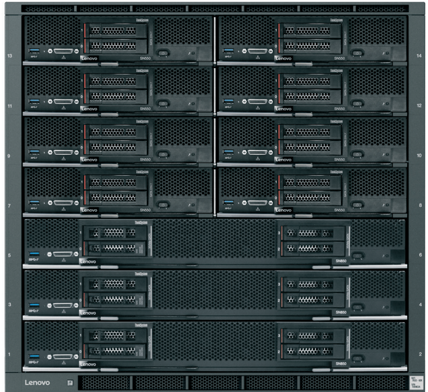
The Flex System Enterprise Chassis houses up to 14 SN550 compute nodes, delivering high density.
