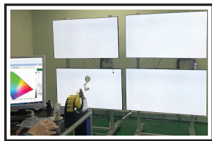
Factory tuning color calibration of white balance
