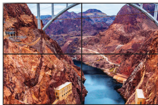
After calibrate and fine tuned white balance
