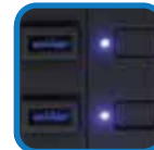
Individual Power Switch with LED Indicator
