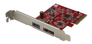
This combination PCI Express controller card lets you add both a USB 3.2 Gen 2 port and an eSATA port to your desktop PC, through a single PCIe slot. The versatile controller card offers a cost-effective way to add high-performance connectivity to your computer, with support for newer USB 3.2 devices as well as eSATA hard drives.
