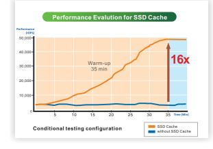
\* SSD Cache speeds up read performance by up to 16 times for frequently-accessed data stored in the cache pool. \* Actual performance gains can vary depending on customer applications.
