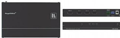
The VM3H2 is a 1:3 distribution amplifier for up to 4K@60Hz (4:4:4) HDMI 2.0 signals, complying with HDCP 2.2 content protection standard. The unit takes one HDMI input, equalizes and reclocks the signal and distributes it to three identical outputs
