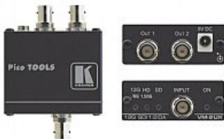
The VM2UX is a compact and highperformance 1:2 4K distributor for standard broadcastgrade SDI signals of up to 12G transmitted data rate. It autoadapts to data rate of one SDI input signal, equalizes and reclocks the signal to improve transmitted signal reach, and distributes the signal to two identical SDI outputs
