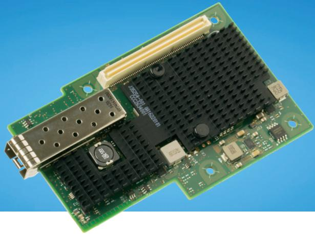
**10/25GbE Open Compute Project (OCP) adapters provide ultimate flexibility and scalability for Cloud and Data Center deployments.**
