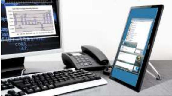
Designed with a piano-black glossy finish, this USB monitor has a 15.6" diagonally viewable image. The I1659FWUX offers a 700:1 contrast ratio, 11 ms response time, and a beautiful 1920x1080 Full HD resolution at 60Hz.
