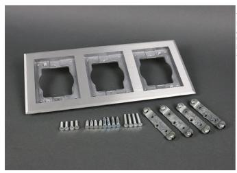
Three gang brushed aluminum combination carpet and tile flange, for OmniBox® and Modulink™ Series floor boxes. Flange is 5.940 inch x 13.170 inch (150.9mm x 334.5mm). Accepts Ortronics MAB6TJ TracJack and MAB3S2 Series II, and Wiremold CM Series Open System adapters, sold separately. NOTE: Brushed aluminum flanges come with beveled edges. Brass cover plates can only be used with brass flanges. Brushed aluminum flanges come with beveled edges.
