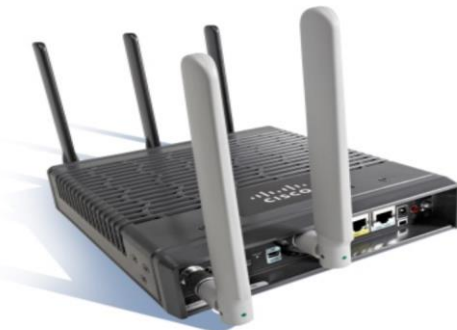
Figure 2. Non-hardened Cisco 819GW Integrated Services Router with 3G and Wi-Fi
