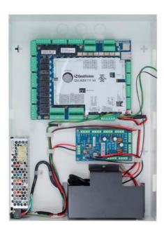
GV-AS4111 Kit is a cabinet containing a GV-AS4111, a power adapter board, a power supply and a casing for backup battery. The power supply provides power to GV-AS4111 Kit and up to 8 output devices (12V, 0.5A per device).
