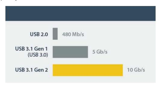
Access and back up your data, faster than ever, by using USB 3.1 Gen 2 technology to leverage the high performance of the latest SSDs and hard drives. This versatile adapter supports data transfer rates of up to 10Gbps - twice the speed of USB 3.0 (USB 3.1 Gen 1) technology.
