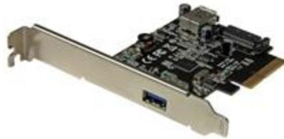
This USB 3.1 Gen 2 card prepares you for the next generation of USB performance, on the inside and outside of your computer. The 2-port card adds one internal Type-A connector as well as one external Type-A connector to your desktop computer, with a combined bandwidth of up to 10Gbps. For power-hungry devices, the card also has an internal SATA power connector, enabling you to use your computer's power supply to add more power to the ports.
