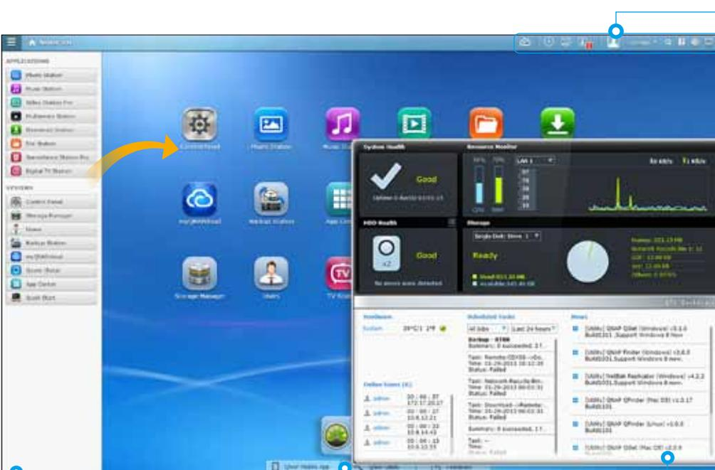
The screenshot shows the QTS 4.1.3 OS desktop. On the left is a vertical 'Main menu' with categories like Applications, SYSTEM, and Services. The desktop has several application icons. A 'Smart toolbar' is at the top right. A 'Smart dashboard' is overlaid in the center, showing system health, HDD status, and network information. A 'Quick search' icon is at the bottom right.
