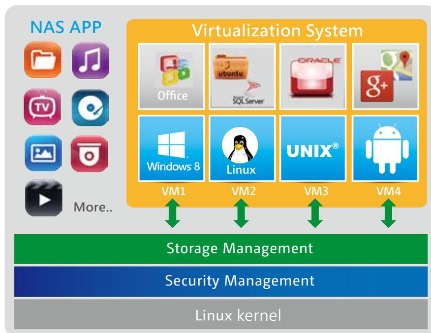
Virtualization technology is normally used in enterprise IT environments, but with the growing needs of a digital office, virtualization is now our everyday applications. Many offices have printers, and when users want to print the documents stored on their Turbo NAS and realized that the printer requires a Windows-only driver, they will need to boot up their PC just for this simple task.
