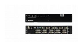
The K244E is a secure 4-port, DVI-I dual-display KVM switch. It provides the highest possible isolation between four connected computers each having two video output ports. The video ports support various video interfaces, from VGA to dual-link DVI and HDMI. Each computer may connect to up to two independent displays and operate in dual-display mode. An RDC port enables user-friendly, comfortable remote control of the KVM switch.
