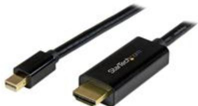
This 6-foot Mini DisplayPort™ to HDMI® adapter cable offers a single-cable connection from your mDP equipped MacBook or Ultrabook™ laptop to an HDMI display or projector. The passive adapter supports video resolutions up to Ultra HD 4K and is Thunderbolt™ compatible when connected directly to a supporting DisplayPort over Thunderbolt I/O port.
