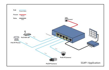
of a PD (Powered Device). The switch will be able to determine if power is to be supplied to any of the PoE supported ports. This helps in the reduction of power used by the switch to power unused ports as well as insuring that power is not put out on wiring that is not connected to a PD.
