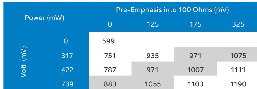
Figure 1 - Power Dissipation (mW, maximum) vs. Rx Output Conditions
